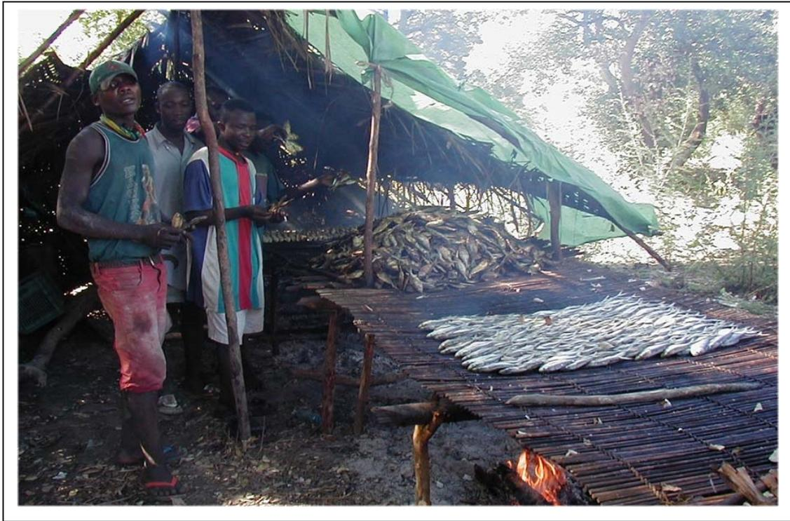
**Plate 7: Traditional smoking kiln, Kibanjo. Note the green plastic sheeting used here to help reduce smoke loss and improve weather proofing.**
